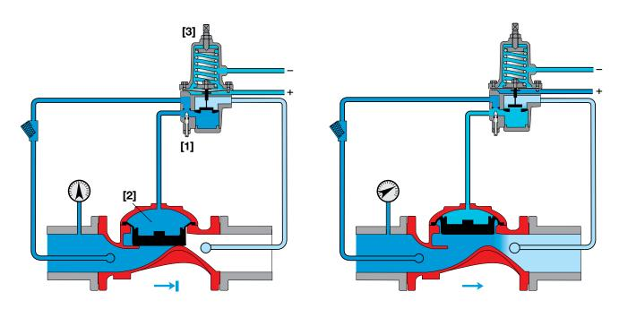
Valve Closed (static condition)
