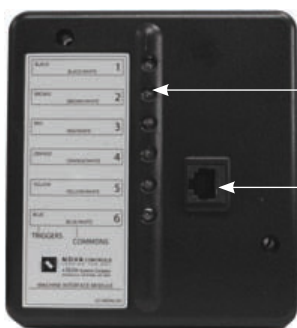
Figure 2-1 Machine Interface LEDs and J2 Cable Connection
