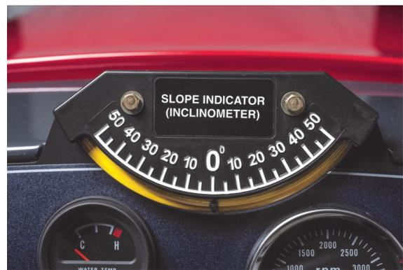
Integral tilt meter fitted as standard
