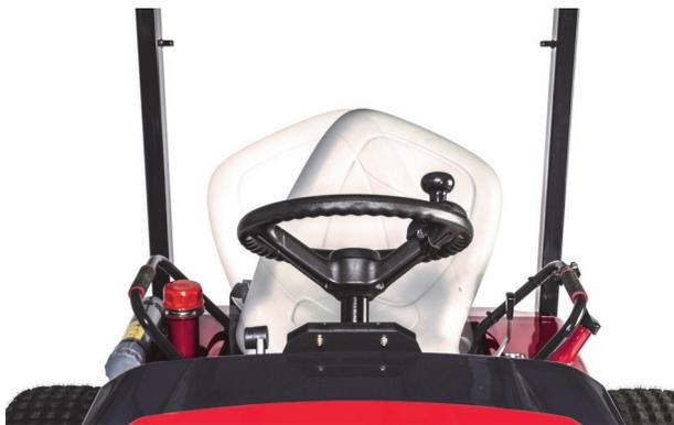
30 degree tilting seat fitted as standard
