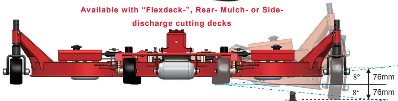
The contour "Flex-deck" prevents scalping and uneven cutting
