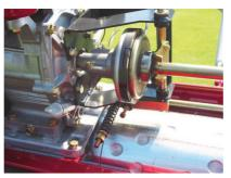
Single plate friction clutch for smooth pickup, precise control and easy engagement of the all-gear drive
