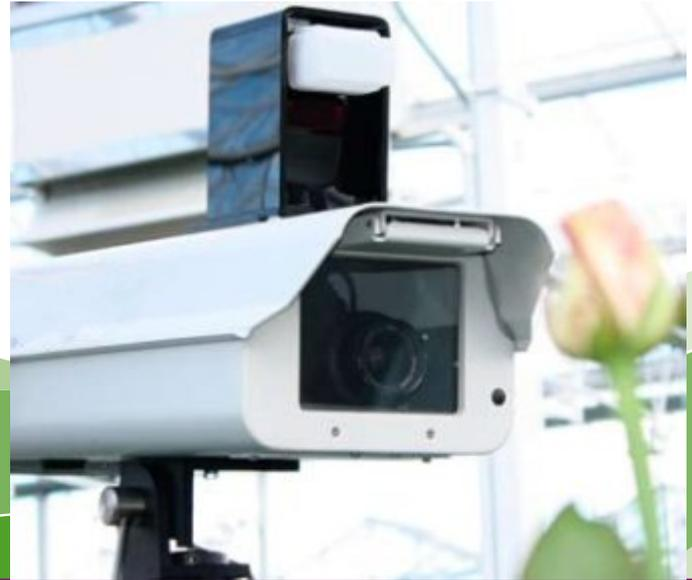
**CropView is a unique solution that allows you to keep track of your crop's development. CropView combines modern digital photography and computerised environmental control, so you can analyse both your crop's current condition and its growth over time. This is all done in unrivalled detail, and available whenever and wherever you want. In-depth field tests have already shown that CropView can result in substantial cost savings in both ornamental and vegetable production.**
