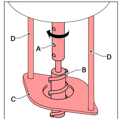
The depth of the hole depends on the position of the drill, which is adjustable. Adjust the depth by placing drill (B) in drill shaft (A).
